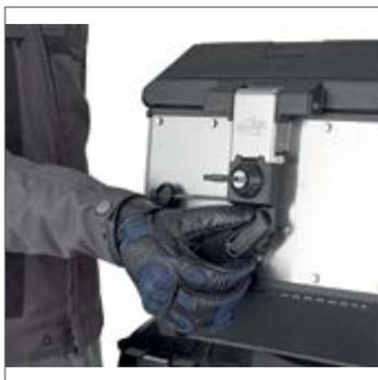
The topcases are released from the plate by turning an external knob that is equipped with a cable system (Patented), placed directly under the Security Lock. It is not necessary to turn the knob to attach the cases
